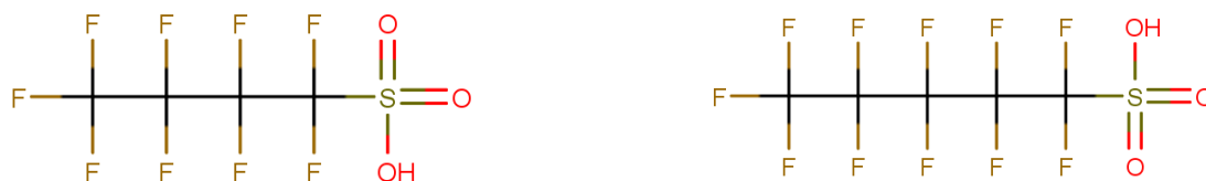
Figura 20: a sinistra, acido perfluorobutan solfonico (PFBS). A destra, acido perfluoropentan solfonico (PFPeS)
